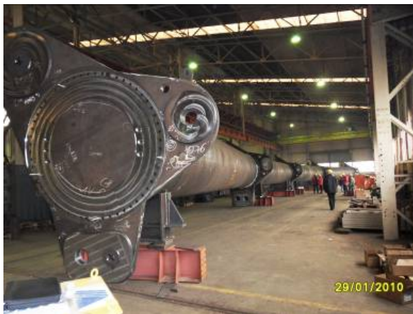
Fig. 8. Trial assembly of the compression ring
