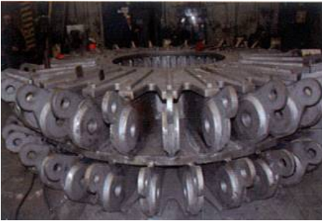
Fig. 5. Central knot, for 60 radial cables fortен (rosette)
