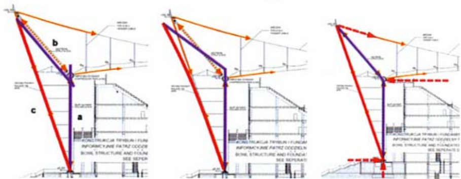
Fig. 4. Triangle of the main pipe elements
